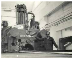
The Schloemann Press for processing aluminium cable installed
