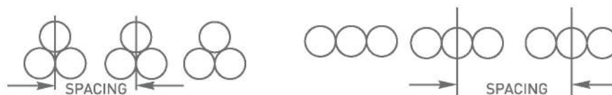
Group Correction Factors For Circuits of Three Single Core Cables in Trefoil and Laid Flat Touching, Horizontal Formation (Average Values)
